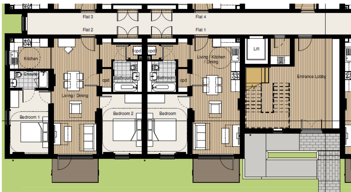
Fig. 2: A Typical layout of one and two bed modules (part-ground floor shown)
